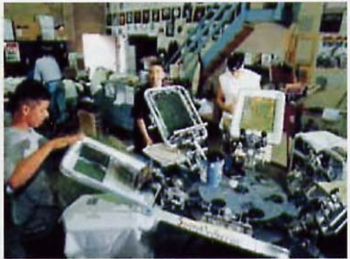
Red blue, yellow, black—each color is applied separately on T-shirts made by youth learning silk-screen skills at Barrios Unidos Productions. A $100,000 loan from the ELCA helped buy equipment.
